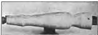
Fig. 130. Tool Handle Roughed.
